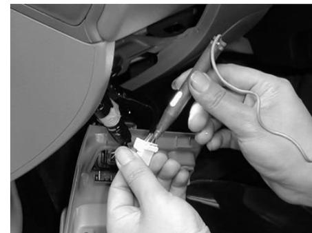
8. Mount Inverter dimmer switch in convenient location and connect to instrument lighting 12volts (red color) connect to ground (black wire) Use a voltage meter to probe for 12V instrument power voltage. We recommend having your headlights 'on' and keys NOT in ignition while probing for the 12 volts instrument lighting. Verify you have found correct wire by turning 'Off' your headlights. With headlights 'off' voltage should be 0 volts.
