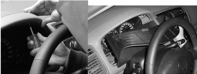
1. Remove plastic trim around instrument cluster. (usually a couple Phillips screws under the top edge) Be careful not to force it. Some cars have Phillips screws hidden under control switches. If you notice the plastic hangs up in a certain area look carefully for control switches (ie defrost button, high beam button etc)
