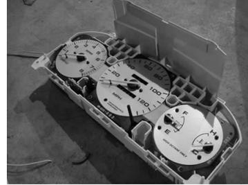
Make sure dials DO NOT rub on pointers in any way. If rubbing occurs make sure dials are centered and bottom of pointer is not rubbing on dial. Replace the stock dial screws.
