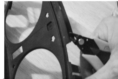
**6. VERY IMPORTANT- Trim any plastic ridges, tabs etc that would interfere (crimp) with the EL panel or wires as it exits the cluster housing.** Not trimming excess plastic away can void warranty. Sharp creases in EL panel can damage it.
