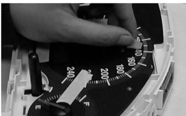
4. Remove stock dial screws (if your car has them) and pull out dial stop pins using pliers (if your car has them) Note: some cars don't have dial screws or dial stop pins For cars that don't have dial screws, place included double-sided tape down on factory dials to hold EL panel in place.
