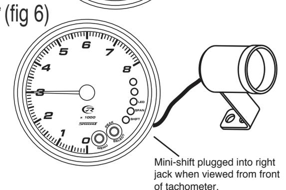
**Note: ONLY plug MINI-SHIFT into tachometer when powered off**
