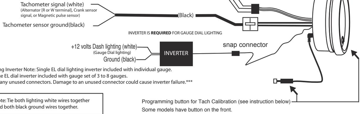
Dial Lighting Inverter Note: Single EL dial lighting inverter included with individual gauge.
