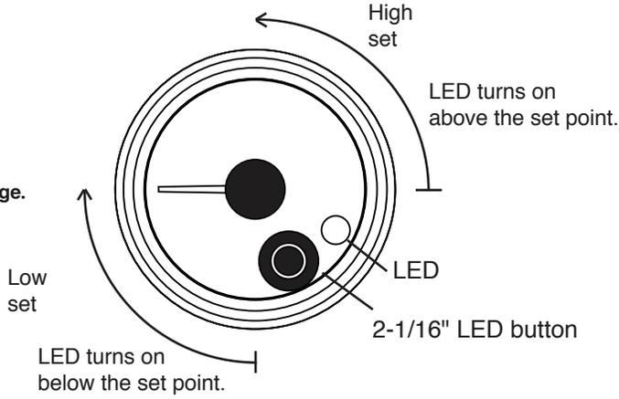
Note: 2-5/8" gauges plug button in back of gauge on **left side only**
